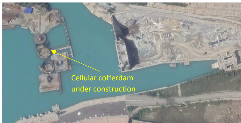
Example of cellular cofferdam construction within the Ghazi Barotha headpond to provide a dry working area for the construction of the 4th Hydropower Extension powerhouse at Tarbela
